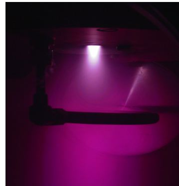
Fig. 2. Picture of an expanding Ar plasma from the ETP plasma source. The injecting ring is visible at 7.5 cm from the plasma source exit.
