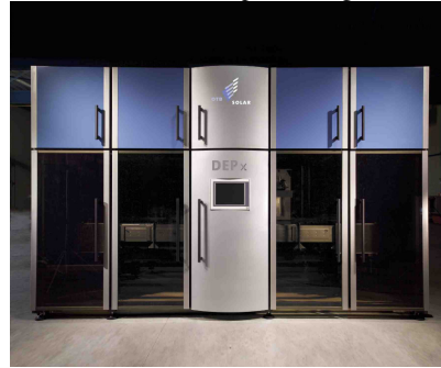
Figure 1: The DEP x , the industrial PECVD tool developed by OTB-Solar employing the expanding thermal plasma technology. This reactor features a high throughput of 960 wafers/hour and a small footprint of 12 m 2 . The reactor can be used for inline as well as for batch wise solar cell production [6].
